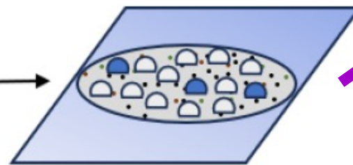
Water droplets are placed directly onto the filter on the glass slide
